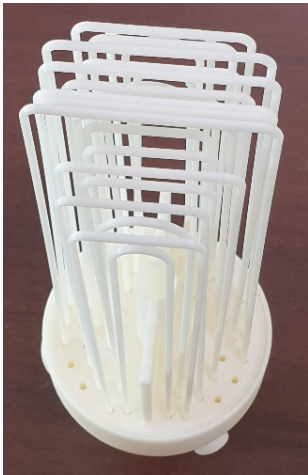
SG – Heat Transfer Pipes (U-tubes)
