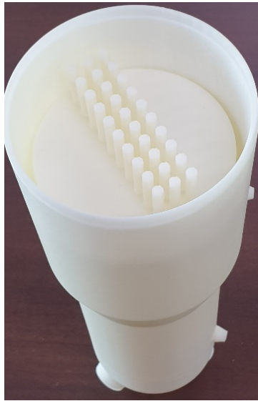
SG – W/O Deaerator (showing Steam Separator)
